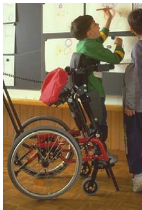
Figure 3: Levo Kid from Levo USA is a child's standing wheelchair.
