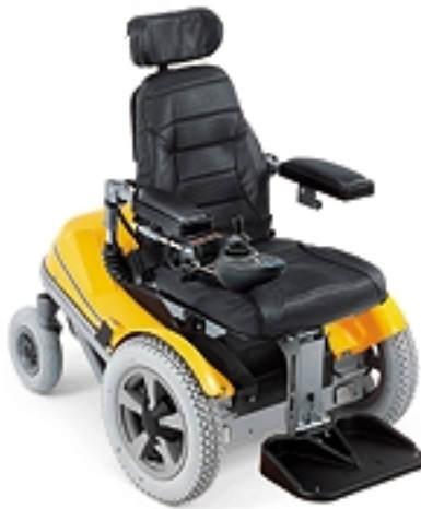
Figure 5: The Chairman Koala Miniflex from Permobil is a child's powered wheelchair.
