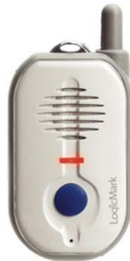
Figure 2: The transmitter for the LogicMark Guardian Alert 911 system. This pendant offers a speakerphone over which a person can speak directly to a 911 operator.
