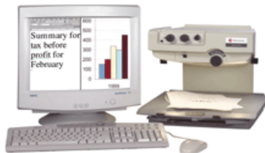
The Aladdin Genie Pro from Telesensory (right) is shown using a split screen to display a graph from the paper on the right half of the computer monitor and text typed into a word processing program on the left side of the screen.
