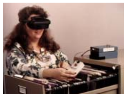
The Magni-Cam from Innoventions is an example of a mouse-style magnifier that can be used with a variety of displays, including a goggles-style display (shown).
